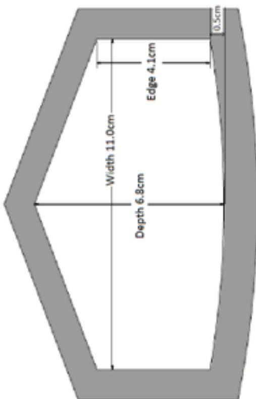
Note: The curve of the lower edge of the aperture is an arc of a circle of radius 12.0 in/30.5 cm, whose centre is on the vertical centre line of the aperture.
